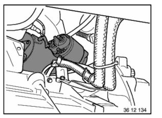
Remove starter in downwards direction. Remove starter motor from crown wheel.
