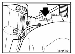
Position of upper screw: Between suction unit and firewall. Remove guide tube for oil dipstick. Unscrew screw.
