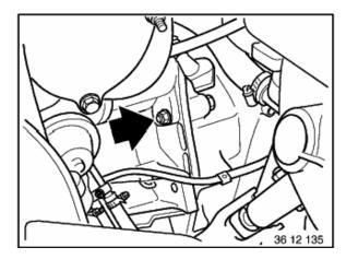
Releasing starter screw, working from below.
